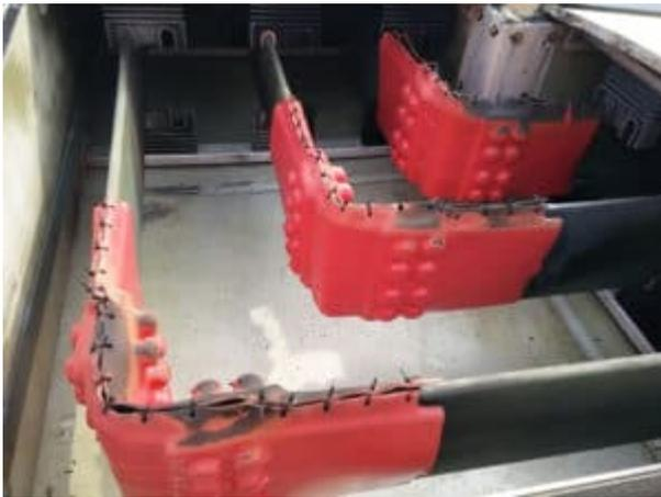
Figure 2: Insulator Boots Burned By Electrical fault
